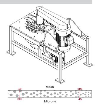
Product Fineness: 50 mesh (300  $\mu$ m)-325 mesh (45  $\mu$ m) Capacity Range: 4-40 TPH
