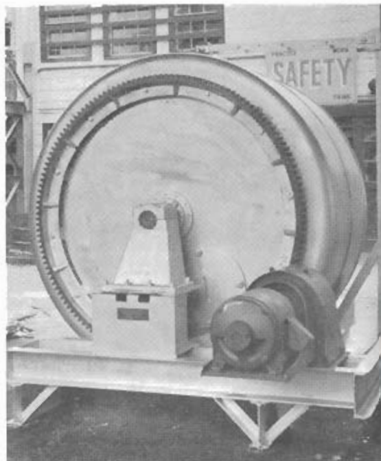
Shown above is one of Sturtevant's rotary dry batch blenders in its final assembly and test running stage.
