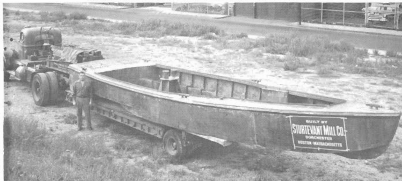
One of the two shallow draft steel vessels constructed by Sturtevant for use in Siam
